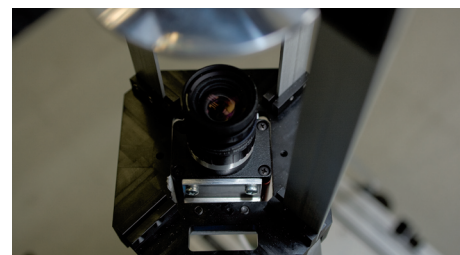
IAISVision: Camera system with omnidirectional mirror
