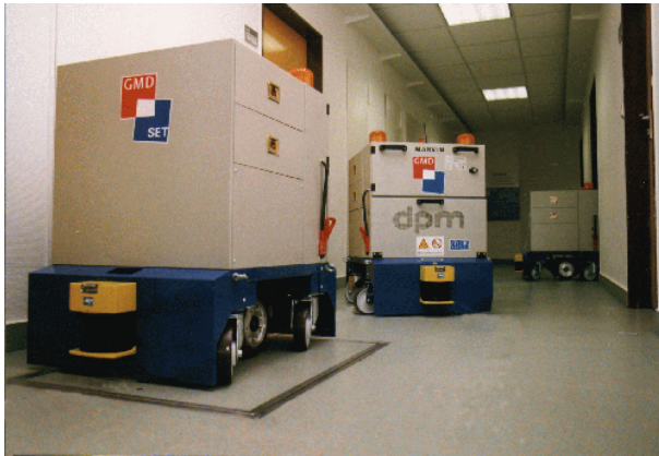
Figure 2: The ARIADNE-team: Odysseus, Marvin, and Thor executing service orders. Each robot is equipped with four drawers, two on each side
