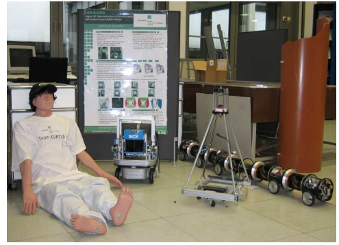
Fig. 4. Complex scene used for a measurement series to determine integration time. Note, that the poster has a glossy surface and quickly leads to oversaturation for short distances.
