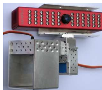
Fig. 1. The Swiss Ranger SR-2 3D camera mounted on a pan-tilt unit.
