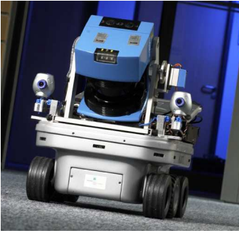
Figure 1: Left: The mobile robot Kurt3D, equipped with a 3D laser scanner based on a SICK LMS-200. Right: Control unit for one motor, based on a feed forward PI controller, thus combines open and closed loop control concepts.
