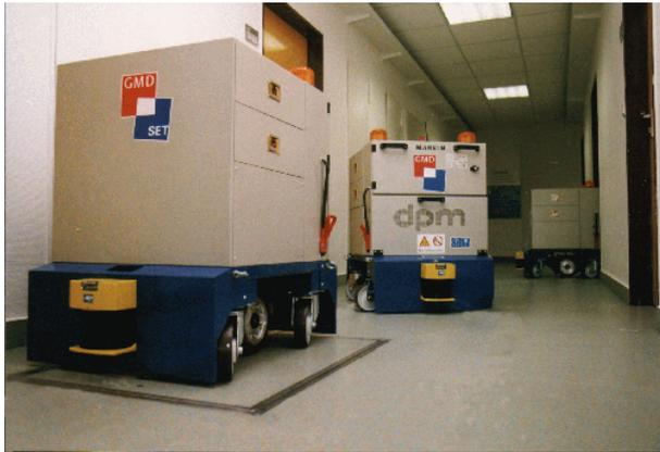
Figure 2: The ARIADNE-team: Odysseus, Marvin, and Thor executing service orders. Each robot is equipped with four drawers, two on each side
