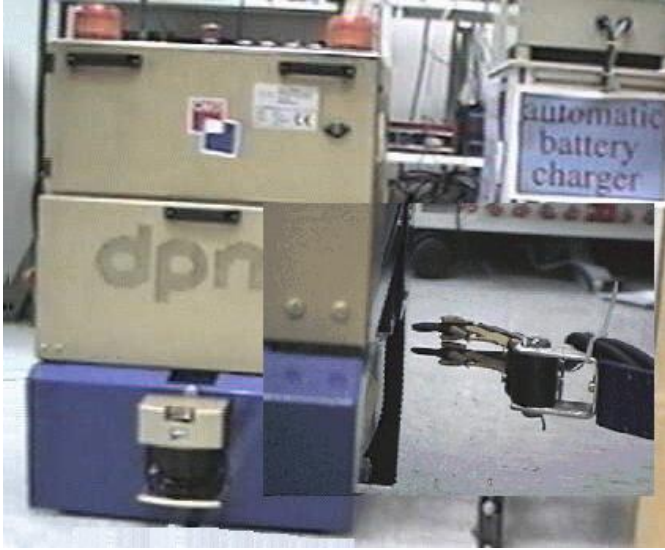
Fig. 1. The robot charging its batteries. It is equipped with two drawers on each side
