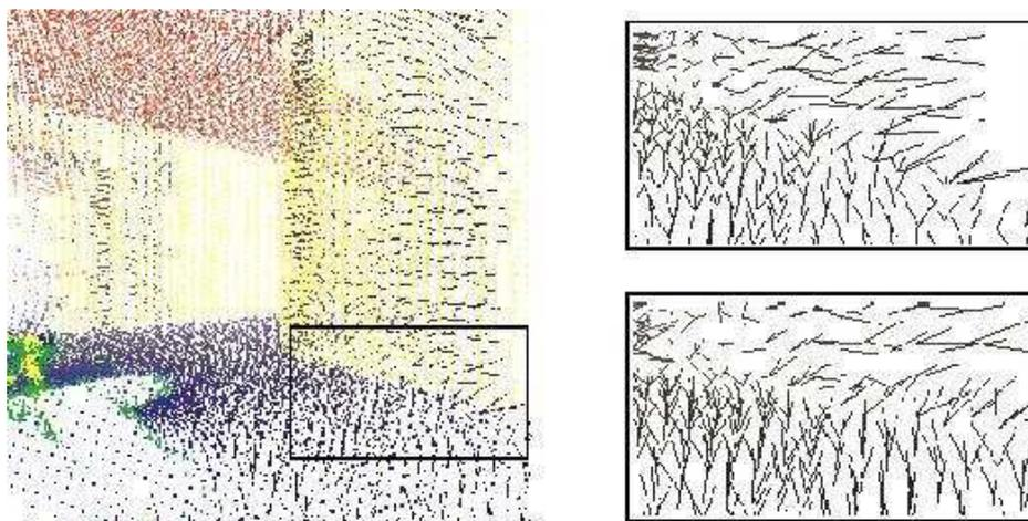
Figure 9: Point pairs for the ICP scan matching algorithm. The left image shows parts of two 3D scans and the closest point pairs as black lines. The right images show the point pairs in case of semantically based matching (top) whereas the bottom part shows the distribution with closest points without taking the semantic point type into account.
