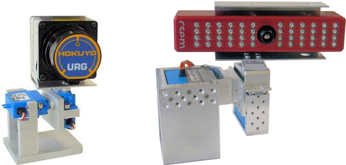
Figure 1: Lightweight Hokuyo laser scanner (left) and CSEM Swiss Ranger (right), both mounted on a pan and tilt unit
