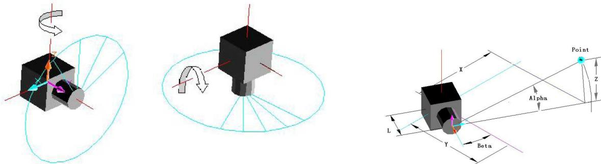
Figure 3: Left: Scanning around the vertical axis to obtain  $340^\circ$  scans of the environment. Middle: Scanning around the horizontal axis to get 3D data in front of a robot. Right: Calculation of the 3D data while turning with the pan/tilt unit.
