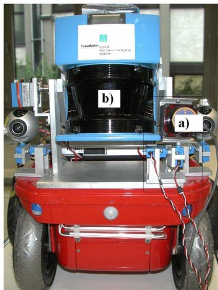
Figure 2: Comparison of the lightweight 3D scanner a) with the bulky 3D-scanner b) as used in RoboCup Rescue on the mobile robot KURT3D.
