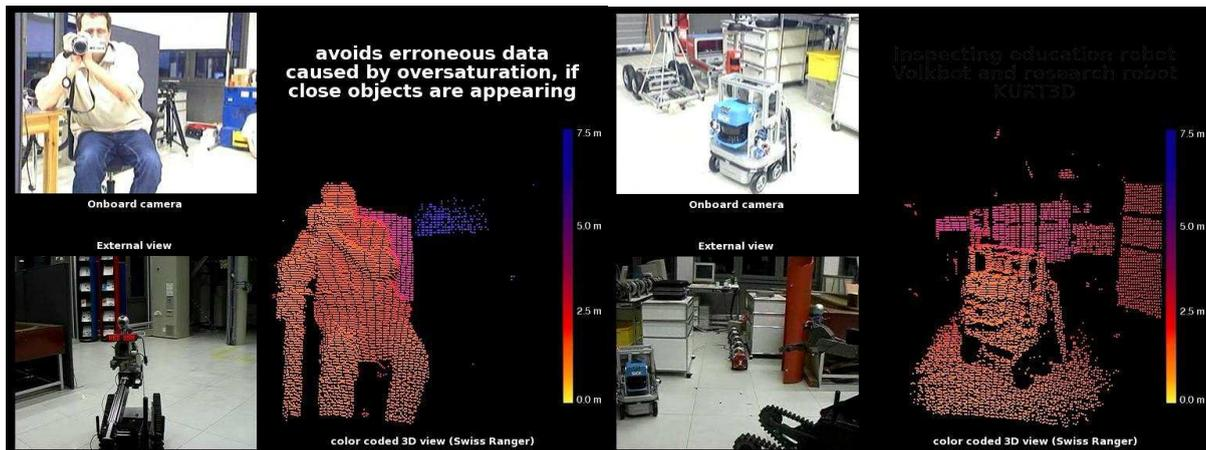
Figure 4: 3D information provided by the Swiss Ranger camera based on the camera calibration and online integration time adaptation / filtering.<sup>1</sup> To illustrate 3D data in this paper, we choose a false color representation using the HSV model starting at 60° in reverse order to 240°. Near objects will appear yellow, far objects blue. Objects with medium distances appear red or magenta.
