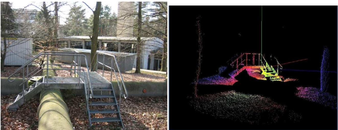
Figure 6: Left: Sewer pipe network at Fraunhofer Campus Birlinghoven. Right: Scanning result displayed by 3D viewer.
