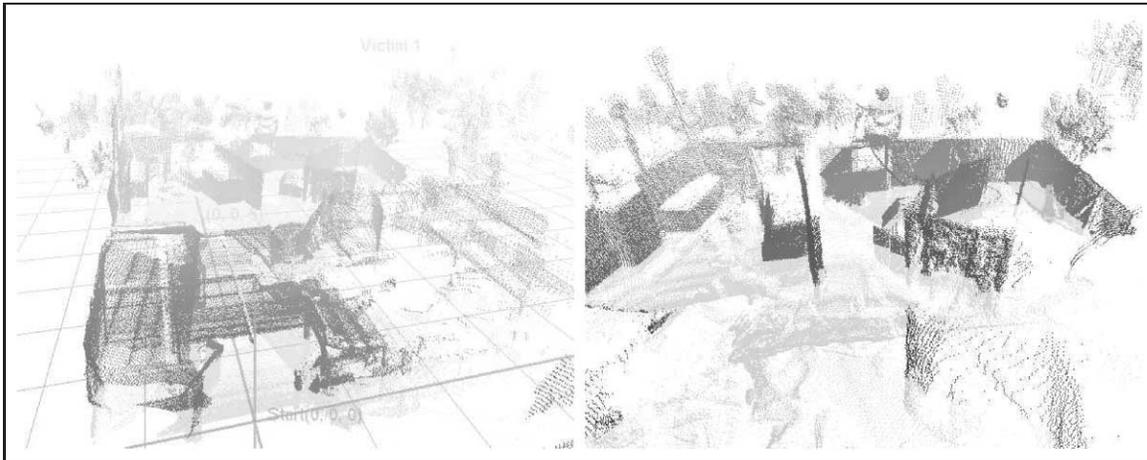
Figure 14 A 3D view of the map of Fig. 13 rendered from a pose slightly above the arena. A  $1\text{ m}^2$  grid is superimposed in the first map.
