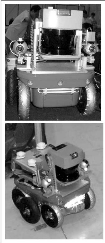
**Figure 1** The mobile robot Kurt3D equipped with the 3D laser range finder as presented at RoboCup 2004. The scanners technical basis is a SICK 2D laser range finder (LMS-200).
