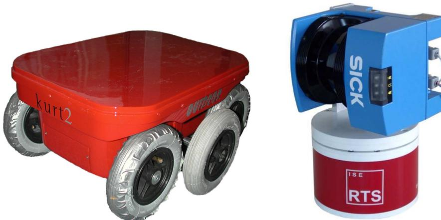
**Fig. 1.** Left: The mobile robot platform Kurt3D outdoor version. Right: . The 3D laser scanner. The scanner rotates around the vertical axis. The technical basis is a SICK 2D laser range finder (LMS-200).
