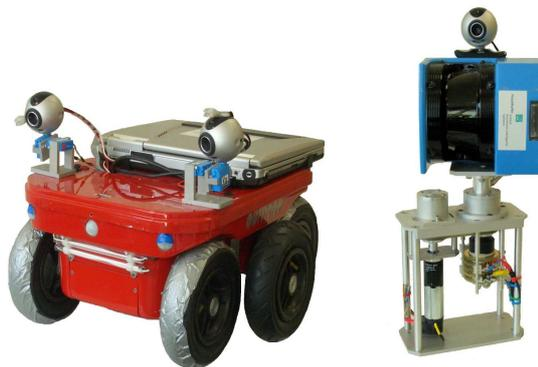
Fig. 1. The tele-exploration robot platform Kurt3D. Left: The six wheel platform with two pan-tilt cameras, illumination and Pentium Notebook. Right: The continuous rotating 3D laser scanner which is based on a standard 2D Laser Range Finder, a SICK LMS200. On top of the scanner a camera is mounted which creates a surround view of the scanned environment.
