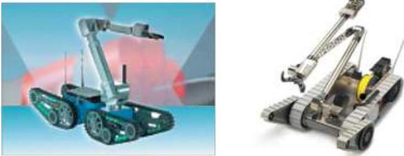
Fig. 2. Left: The teleMax robot system from teleRob [2]. Equipped with a 7 DOF manipulator and 3 cameras. The flippable four-track drive ensures maximum mobility. Right: The PackBot EOD system from iRobot [1]. Also a flippable four track drive but with another setup. Designed to be carried by one person only and equipped with a manipulator and cameras.
