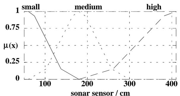
Figure 5: Membership functions for the sonar sensors
